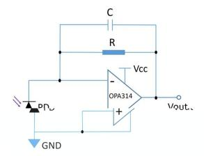
$V_{out}(V) = I_{ph}(A) \times R(\Omega)$
